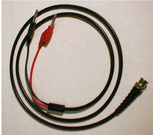
Figure 14. Cable for connection of voltmeter to the ODU RSSI port
